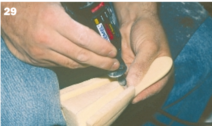
29. Again, it is easier to use a Dremel grinder to remove where the lower jaws will be placed.
