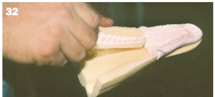
32. Align each jaw side with the front palate and check to see if everything is matching correctly. If not, remove or add material wherever needed to achieve proper alignment.
