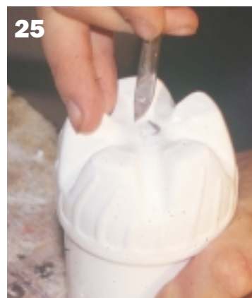
25. Let the RTV cure and then remove the water bottle. The RTV will have different curing times depending on it you are using fast, regular or slow setting RTV. I like to let the RTV cure a little longer than recommended to be sure that everything is full set. If you open the mold before everything is set, the mold will be ruined. In this photo you can see that I am using a scalpel to cut the RTV rubber a way from the base of the tongue. The hole that I am creating will help remove the tongue from the mold and provide a pouring hole when it is time to cast the tongue.
